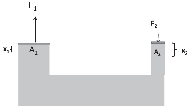
Figure 20.5 A hydraulic press that amplifies the force is made of two cylinders of different cross-sectional areas A_1 and A_2 , connected by a horizontal segment. Given P_2 = \frac{F_2}{A_2} = \frac{F_1}{A_1} = P_1 , the equality of the pressures, and A_1 x_1 = A_2 x_2 (the equality of volumes displaced in the two sides), we find \frac{F_2}{F_1} = \frac{A_2}{A_1} = \frac{x_1}{x_2} . A small force F_2 acting on the right cylinder pushes the incompressible fluid by a distance x_2 , and this leads to large force F_1 on the left that moves the piston over a smaller distance x_1 . Energy is conserved because F_1 x_1 = F_2 x_2 , as in a lever.
